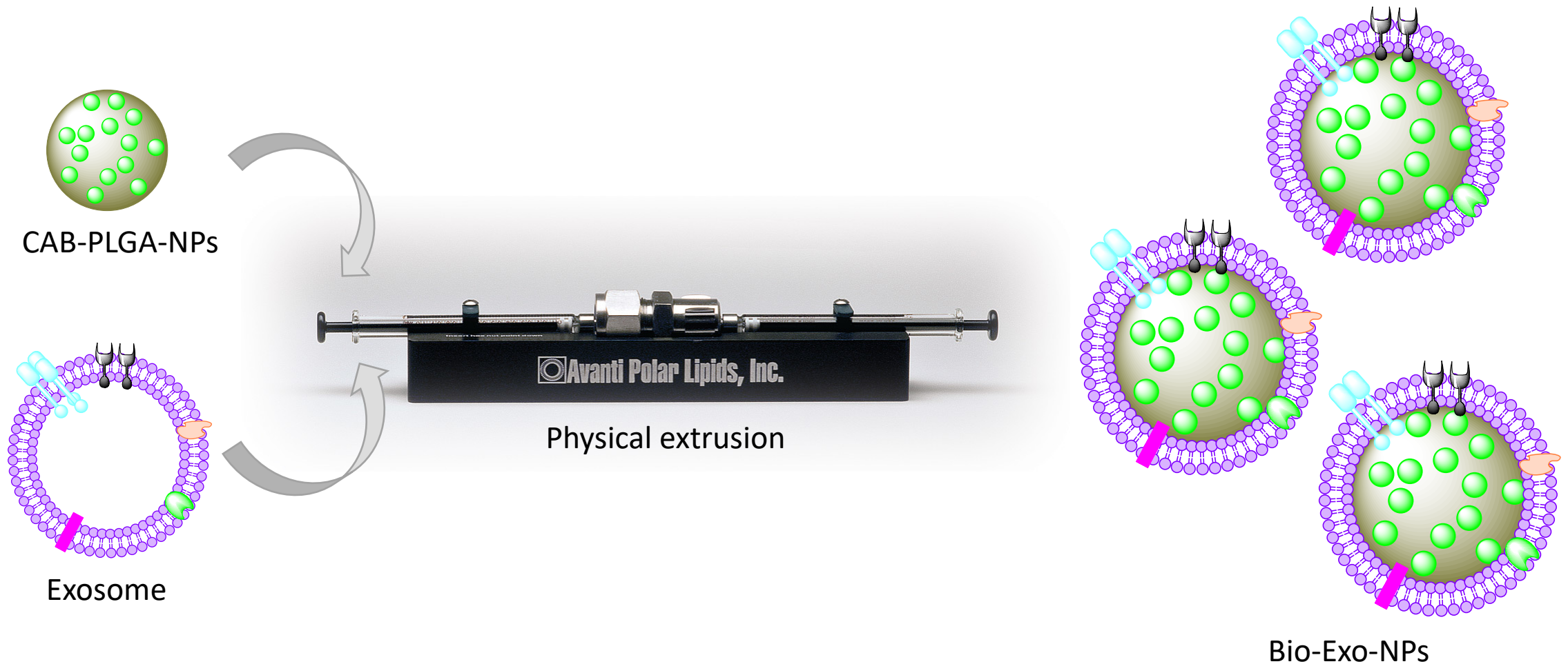
Schematic of exosome coated PLGA NP preparation by Co-extrusion methods
