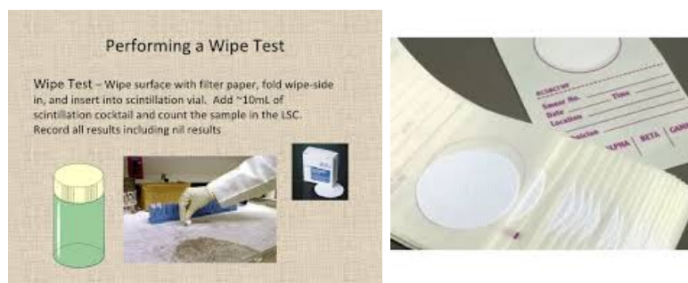
Figure 5 Wipe test procedure and wipe test plate
