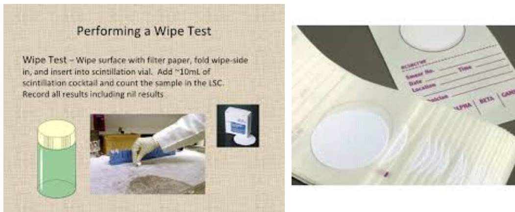
Figure 5 Wipe test procedure and wipe test plate
